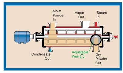
temperature and avoids thermal degradation of heat sensitive materials. An adjustable weir at the discharge end controls the level and quantity of solids in the dryer between 25% and 75% full. You control the residence time in the dryer by adjusting this weir or the feed rate.
