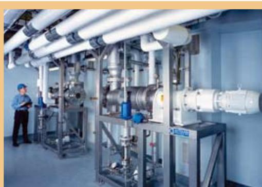
5 sq. ft. Artisan Rototherms® used for solvent recovery at a cGMP facility.
