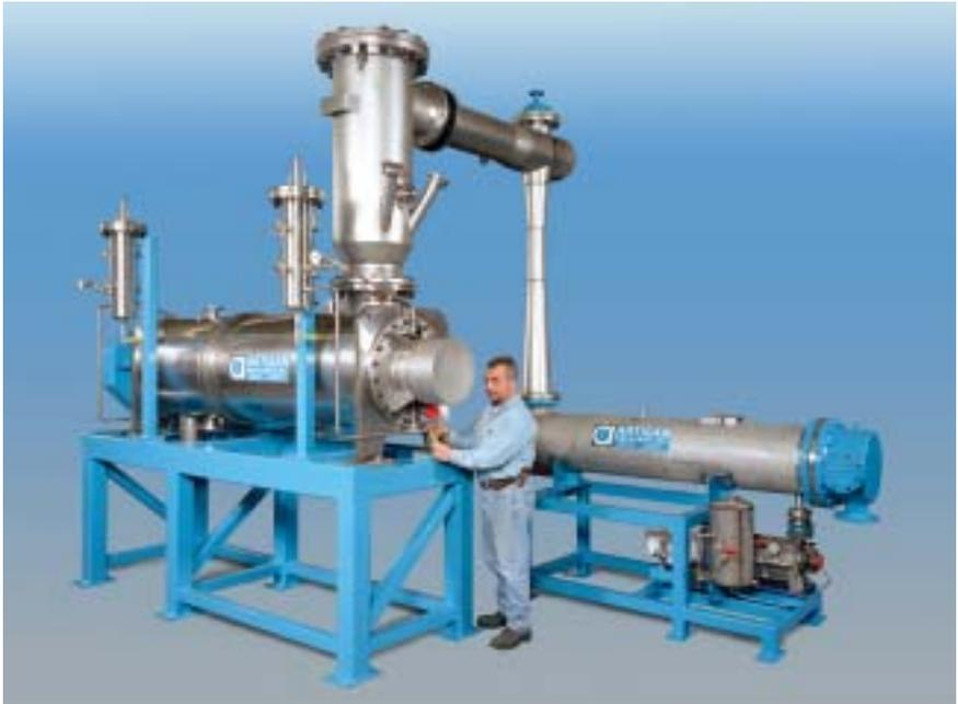
20 sq. ft. Rototherm® with Jet-Vac® hybrid vacuum system. This Rototherm concentrates and produces free-flowing powder for the food industry.
