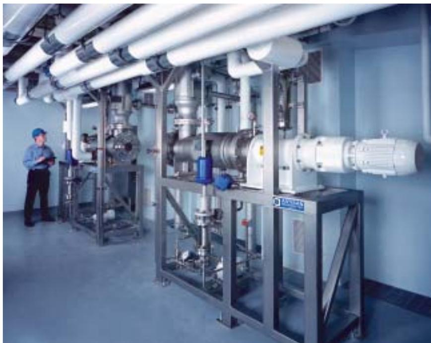
Installed in a cGMP facility, this Rototherm is designed to purify API, intermediates or fine chemicals.
