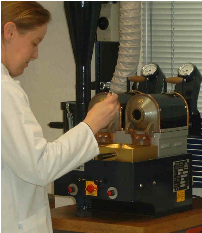
Battery sample roaster, type BRZ 2
